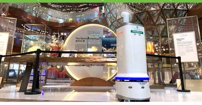
GF Technoavation's VirusGuard is equipped with a nozzle-spray system to thoroughly disinfect large spaces effectively and efficiently, with disinfectants lab-tested to be safe for humans.
